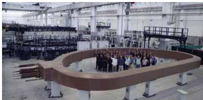
One of ITER superconducting toroidal field coil built in Italy, ready to ship to ITER. © Let there be Light.
