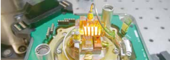
Figure 4. A quantum memory based on a Europium-doped crystal. The crystal is mounted inside a closed-cycle cryostat that cools it to about 3 K. Multiple photonic qubits can be stored inside this crystal for durations of up to one millisecond.
